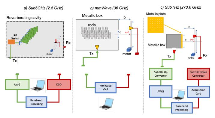
Figure 1. The designed experimental setups for the investigation of the spatiotemporal focusing capability of TR-based wireless communications centered around the considered carrier frequencies: (a) 2.5 GHz, (b) 36 GHz, and (c) 273 GHz. Detailed descriptions are provided in Section III-A.
