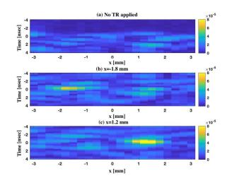
Figure 4. The TR spatiotemporal focusing capability of the subTHz system in Fig. 1(c) operating at 273.6 GHz with bandwidth B = 3 GHz for different Rx positions. The received signal strength without applying TR is also sketched.
