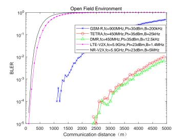
Fig. 2. BLER performance in open field environment with a single antenna and without retransmission when the physical layer parameters are specified in the standard.
