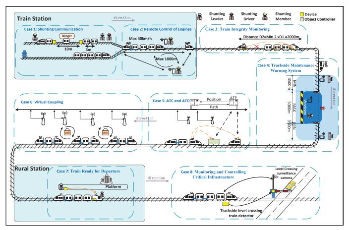
Fig. 1. Use cases of off-network communication in FRMCS.
