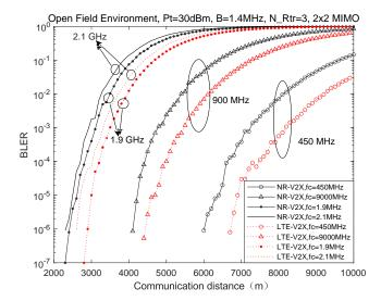
Fig. 4. BLER performance in open field environment with MIMO and retransmission when B=1.4 MHz,  $P_t=30$ .
