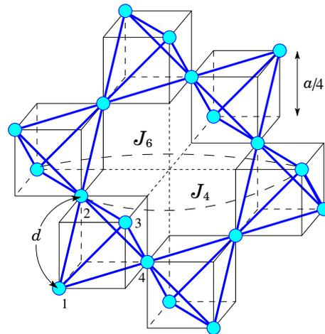
FIG. 1. Crystal structure of cubic spinels  $AB_2O_4$  with B-site cations shown by circles. The relevant exchanges beyond the nearest-neighbor shell are indicated by long-dashed lines. Site indices in a unit cell tetrahedron are shown by numbers.
