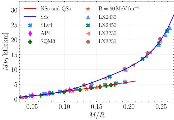
**Figure 8.** Scaled frequency of the  $f$ -mode as a function of the compactness  $C$ . The solid lines represent universal relations in Eqs. (20) and (21).
