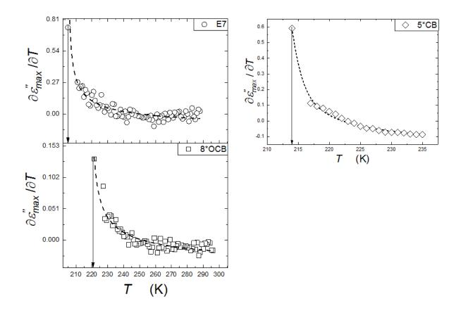
FIG. 2 Derivative-based analysis by Eq. (3) of eps max for studied system. Strong anomaly occurs near glass transition temperature.
