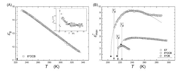
FIG. 1 (A) Static dielectric permittivity of 8\*OCB liquid crystal in isotropic phase near  $T_g$ . (B) Pretransitional anomaly in the vicinity of glass transition for all studied system. Dashed lines denote relation (2). Fitting parameters are given in Table 1.
