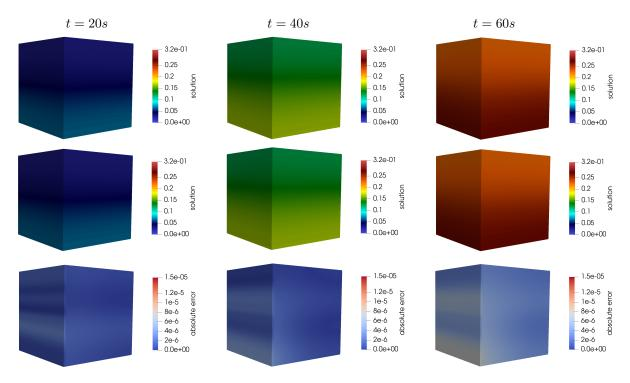
Figure 9: Slave solution FOM (top), ROM (center) solutions and absolute error (bottom) for  $\alpha=2.75$  and three different time instants.
