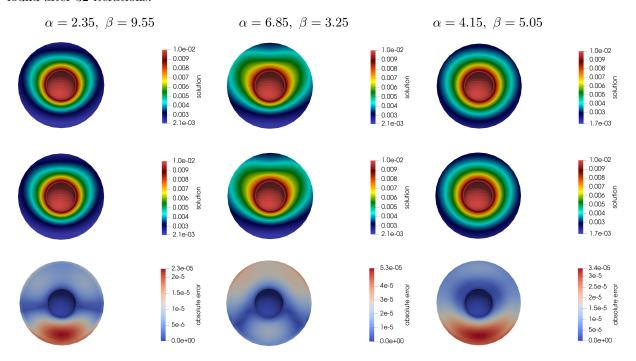
Figure 5: Slave solution FOM (top), ROM (center) solutions and absolute error (bottom) for three different parameter vectors.
