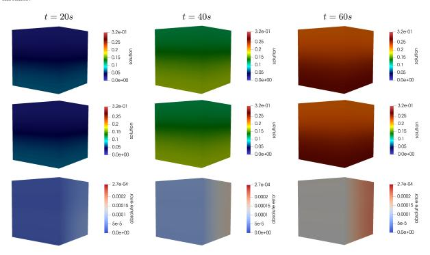
Figure 10: Master solution FOM (top), ROM (center) solutions and absolute error (bottom) for  $\alpha = 2.75$  and three different time instants.
