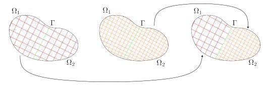
Figure 1: Schematic representation of the two discretizations of the domain  $\Omega$  used to compute the FOM snapshots (left and center) and the discretization of the domain  $\Omega$  used to compute the ROM snapshots (right).
