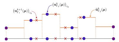
Figure 3: Geometrical interpretation of the interface reduction with the DEIM. The blue points represent the magic points on  $\Gamma_2$  and the values of  $\mathbf{u}_{\Gamma_2}^k$  at these magic points, the orange lines represent the piecewise constant interpolating function  $\tilde{\mathbf{u}}_{\Gamma_2}^k$ , while the red crosses are the magic points on  $\Gamma_1$  and the values of  $\mathbf{u}_{\Gamma_1}^{k+1}$  at these magic points.
