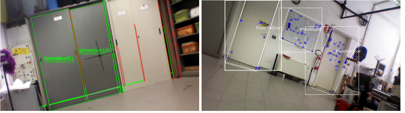
Fig. 1. Two sample frames output of a semantic object detection (left) and tracking (right) system. Tracker uses the CMT algorithm.
