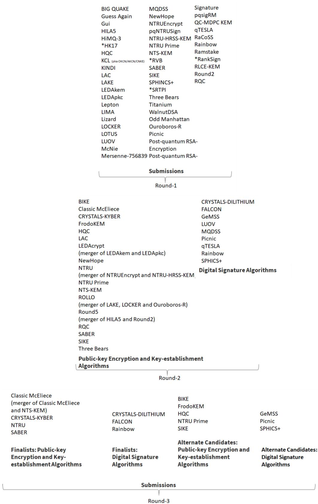
**Figure 2:** NIST Post-quantum Cryptography Algorithm Progresses in 3-Rounds
