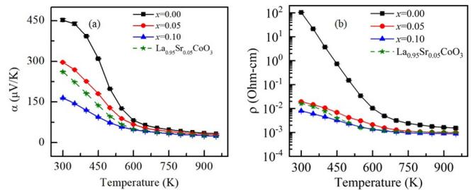
FIG. 2: Figure 2: Seebeck coefficient ( $\alpha$ ), electrical resistivity ( $\rho$ ) as a function of temperature for  $(\text{LaNdPrSmEu})_{1-x}\text{Sr}_x\text{CoO}_3$ .
