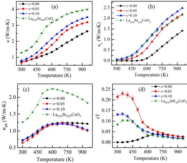
FIG. 3: (a) Total thermal conductivity ( $\kappa$ ), (b) electronic thermal conductivity ( $\kappa_e$ ), (c) phonon thermal conductivity ( $\kappa_{ph}$ ), and (d) figure of merit ( $zT$ ) as a function of temperature for  $(\text{LaNdPrSmEu})_{1-x}\text{Sr}_x\text{CoO}_3$ . A comparison of these parameters for simple perovskite  $\text{La}_{0.95}\text{Sr}_{0.05}\text{CoO}_3$  is also shown.
