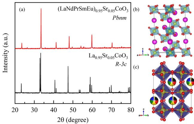
FIG. 1: (a) XRD pattern of  $\text{La}_{0.95}\text{Sr}_{0.05}\text{CoO}_3$  and  $(\text{LaNdPrSmEu})_{0.95}\text{Sr}_{0.05}\text{CoO}_3$  is shown. The crystal structure using Vesta software is shown for (b)  $\text{La}_{0.95}\text{Sr}_{0.05}\text{CoO}_3$ , and (c)  $(\text{LaNdPrSmEu})_{0.95}\text{Sr}_{0.05}\text{CoO}_3$ . The structural parameters are obtained from the Rietveld refinement of the XRD pattern.
