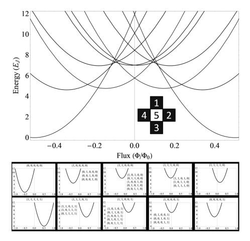
Figure 6: The energies associated with five square plaquettes arranged in a spin star when each contains an odd number of  $\pi$ -junctions.
