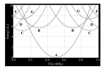
Figure 5: The energies for the triangular Josephson junction triangular array as a function of flux. A  $\pi$ -shift is developed due to the introduction of an odd number of  $\pi$ -junctions in each plaquette.
