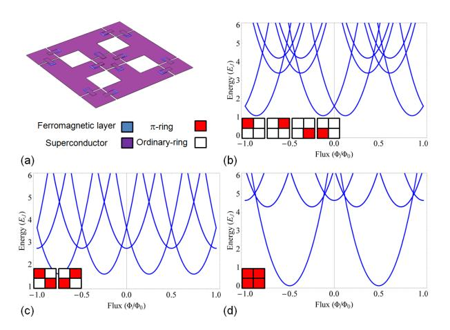
Figure 1: A system composed of superconductor-ferromagnet-superconductor Josephson-junctions [4] with four plaquettes. The total energy is normalised by the Josephson energy as a function of the magnetic flux in the system. The energy is calculated using the quasiclassical method [9].
