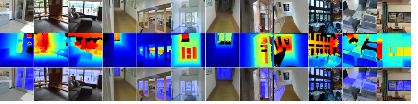
Fig. 2. Examples from our RGB-D GSD dataset. Top, middle and bottom rows show RGB images, depth maps, and GT glass surface masks overlaid on the RGB images, respectively.
