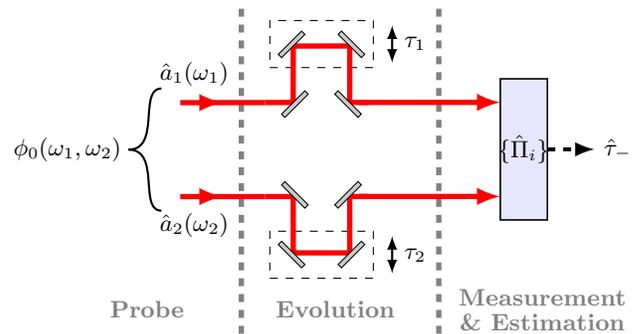
FIG. 1. A general scheme for estimation of the relative photon delay  $\tau_- = (\tau_1 - \tau_2)/2$  using a two-photon probe state. The probe, consisting of a single photon in each of two spatial modes ( $\hat{a}_1$  and  $\hat{a}_2$ ), undergoes delays ( $\tau_1$  and  $\tau_2$ ) in each arm. Measurement(s) are made (depicted by the projectors  $\{\hat{\Pi}_i\}$ ), and the relative delay is estimated from measurement statistics.
