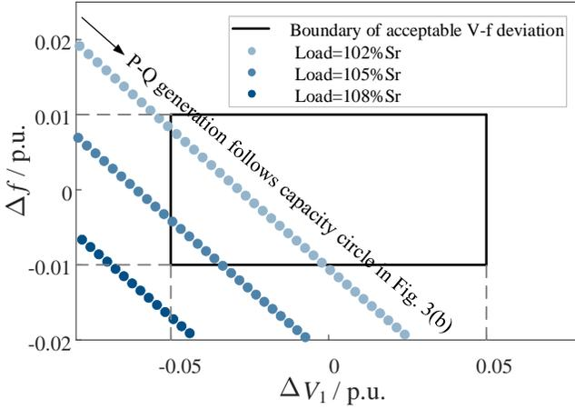
Fig. 6 V-f deviation under bounded generation constraints.
