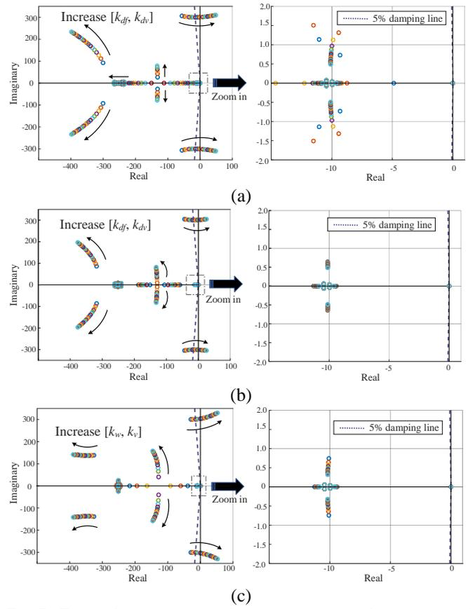
Fig. 7. Eigenvalue trajectories when sweeping control parameters (a) Condition 1: crossing droop gain  $[k_{df}, k_{dv}] = [0.025, 0.125]$ ; (b) Condition 2: crossing droop gain  $[k_{df}, k_{dv}] = [0.0165, 0.0825]$ ; (c) Condition 3: crossing power regulator gain  $[k_w, k_v] = [0.0825, 0.0619]$ .
