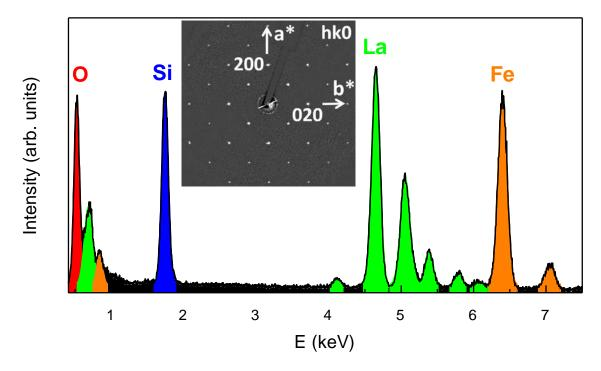
FIG. 1. EDX spectrum recorded on one crystallite showing an oxygen peak at 0.525 keV in the LaFeSi matrix. **Inset:** hk0-cut of the reciprocal space indexed in P4/nmm space group of LaFeSiO<sub>1- $\delta$ </sub>.
