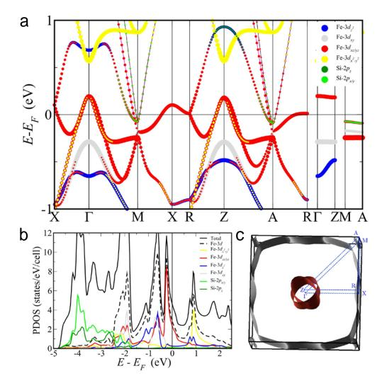
FIG. 5. Calculated electronic structure of LaFeSiO. **a:** Orbital-resolved band structure along the high-symmetry directions of the P4/*nmm* Brillouin zone. **b:** Orbital-resolved density of states. **c:** Perspective view of Fermi surface computed on the basis of the experimental structure in Table I. The labels indicate the high-symmetry points and lines correspond to the *k*-path in **a**
