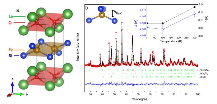
FIG. 2. **a**: The crystal structure as determined by NPD. The structure is shifted by (0,0,0.5) to emphasize the Fe containing layer. **b**: Rietveld refinement of the NPD data collected at 300 K at the D1B instrument of ILL. Three phases are included: LaFeSiO<sub>1- $\delta$ </sub>, LaFe<sub>2</sub>Si<sub>2</sub> and unreacted LaFeSi (from top to bottom). **Inset**: Temperature dependence of *a* and *c* lattice parameters.
