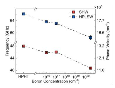
**Figure 4:** Frequency and velocity of surface phonons in diamond as a function of the boron doping concentration. The data for the SHW and HPLSW phonon polarization branches are shown at  $q_{\parallel} = 0.0228 \text{ nm}^{-1}$ .
