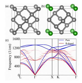
**Figure 5:** (a-b) The supercell structure of the pristine and the B-doped diamond. The grey and green spheres represent C and B atoms, respectively. (c) The calculated phonon band structure of the pristine (blue) and B-doped (red) diamond. The softening of all acoustic phonon modes as a result of boron doping is clearly observed. Note that we assumed substantially higher concentration of B atoms in order to keep the supercell reasonably small in the calculations.
