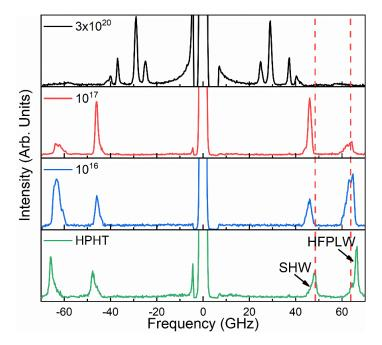
**Figure 3:** Brillouin light scattering spectra of the boron-doped diamond samples and a reference HPHT diamond substrate accumulated at  $\theta = 75^{\circ}$ . The shear-horizontal surface wave and high-frequency pseudo-longitudinal wave are labeled as SHW and HFPLW, respectfully. The frequency of types of phonons decreases as the boron concentration increases.
