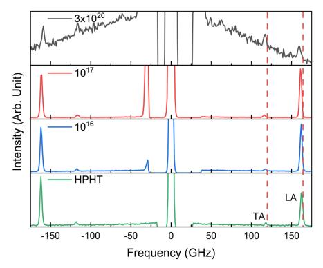
**Figure 2:** Brillouin light scattering spectra of the boron-doped diamond samples in the backscattering geometry performed at a 20° incidence angle. The dashed lines are guides to the eye to illustrate the decrease in the acoustic phonon frequency as the doping level increases. The peaks labeled as LA and TA correspond to the longitudinal acoustic and the transverse acoustic bulk phonons.
