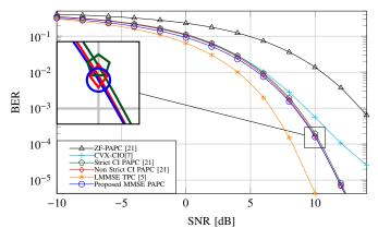
Fig. 3: BER versus SNR for K = 10, M = 30,  $\alpha_s = 8$
