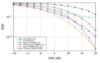
Fig. 2: BER versus SNR for K = 15, M = 15,  $\alpha_s = 4$
