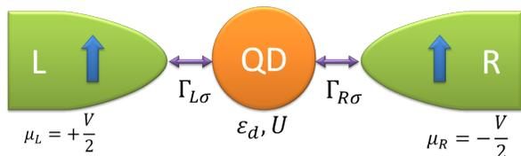
FIG. 1. Model system – A magnetic impurity (quantum dot or molecule), characterized by an orbital level of energy  $\varepsilon_d$  and Coulomb correlations  $U$ , is attached to two ferromagnetic contacts with spin-dependent coupling strengths  $\Gamma_{L\sigma}$  and  $\Gamma_{R\sigma}$ , respectively. These leads are locally in equilibrium at a global temperature  $T$ , yet with a voltage bias  $V = \mu_L - \mu_R$  that is applied symmetrically across them.
