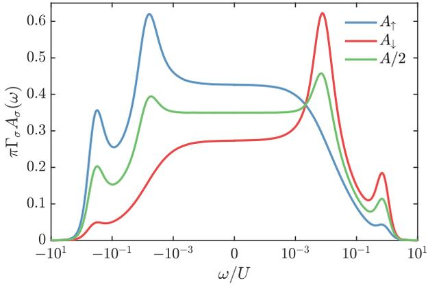
FIG. 7. The energy dependence of the equilibrium zero-temperature normalized spectral function  $\pi\Gamma_\sigma A_\sigma(\omega)$  calculated for  $\varepsilon_d = -U/3$ ,  $p = 0.2$  and  $B = 0$  [Eq. (6)]. The dashed lines show the negative part of the energy spectrum. Note the logarithmic energy scale.
