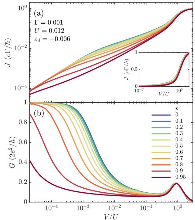
FIG. 2. The bias voltage dependence at  $T = 0$  and particle-hole symmetry  $\varepsilon_d = -U/2$  of (a) the mean current  $J$  on a log-log scale (inset lin-log), and (b) the corresponding differential conductance  $G$  on a lin-log scale. The various curves are for different values of the lead spin polarization  $p$ , as indicated.
