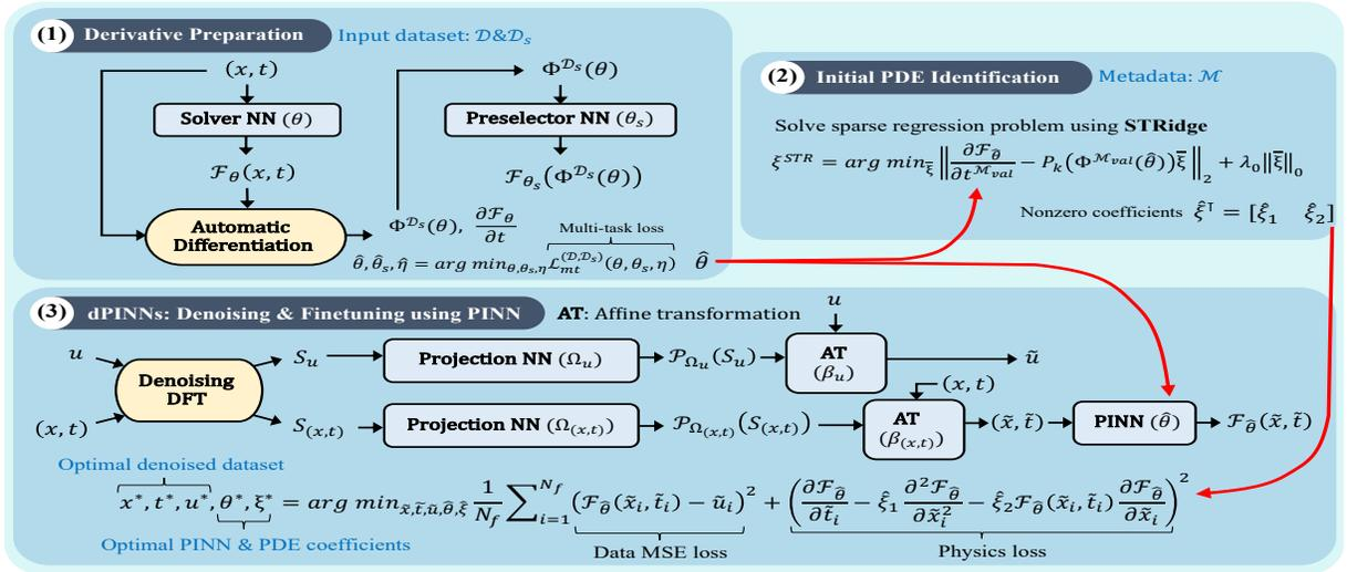
Fig. 1: Exemplary discovery scheme of the proposed **noise-aware Physics-informed Machine Learning (nPIML) framework**: (1) Physics-regularized derivative preparation by multi-task learning of the solver and preselector. (2) PDE identification of the hidden PDE by STRidge. (3) Applying the denoising DFT to  $(x, t) \& u$  then finetuning the initial PDE coefficients on the denoised variables, using PINN.
