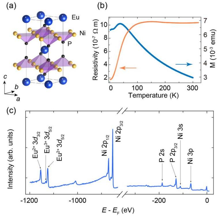
FIG. 1 (a) Schematic illustration of the crystal structure of  $\text{EuNi}_2\text{P}_2$ . (b) Resistivity and magnetization as a function of temperature with magnetic field applied along the  $c$  axis. (c) X-ray photoemission spectrum showing the characteristic  $\text{Eu}^{2+}$  and  $\text{Eu}^{3+}$   $3d$ -doublets as well as Ni and P core levels.
