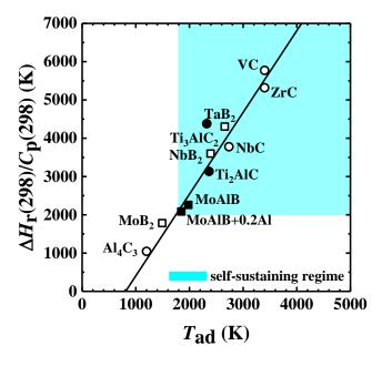
Figure 9 Relationship between  $\Delta H_r(298)/C_p(298)$  (K) and  $T_{ad}$  for selected compounds. Most of Compounds are reported in [41]. Compounds (**•**) (**□**) are the MAB phase and binary borides, Compounds (**•**) (**○**) are the MAX phase and binary carbide. The selfsustaining regime on the right side indicates that the material can be synthesized using the SHS method with  $T_{ad} \ge 1800$  K and  $-\Delta H_r^{298K}/C_p^{298K} \ge 2000$  K.
