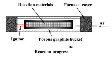
Figure 1 The set-up for self-propagating high-temperature synthesis apparatus.
