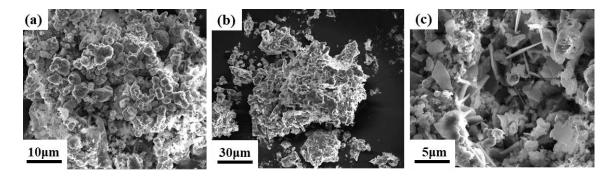
Figure 6 Morphology of samples synthesized from 1Mo/1.3Al/B by SHS for (a) Coarse raw powder, (b)Fine raw powder, and (c) Ultra-Fine raw powder.
