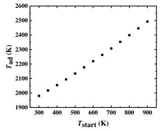
Figure 8  $T_{ad}$  as a function of the starting temperatures ( $T_{start}$ ) for the SHS reaction of Mo + Al + B = MoAlB.
