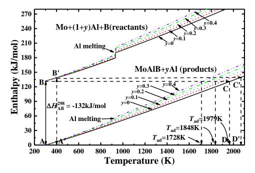
decrease of  $T_{ad}$ , but offers the potential to control the exothermicity of the SHS.
