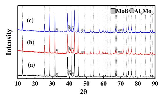
Figure 5 XRD patterns of samples synthesized from Mo/1.3Al/B by SHS with (a) Coarse raw powder, (b) Fine raw powder, and (c) Ultra-Fine raw powder
