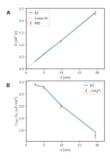
FIG. S9. (a) Total resistance at low frequency as a function of the electrode-electrode distance, as calculated from MD (symbols) and EC models (solid line). The results are compared with a linear fit of the MD results to show the extrapolation at d = 0. (b) Comparison between cell capacitance calculated from MD using the electrode charge fluctuations  $\beta \langle \delta Q^2 \rangle$  (symbols) and from EC models (solid line) for all the considered inter-electrode distances.
