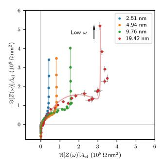
FIG. 3. Nyquist plot of the impedance  $Z(\omega)$  in the complex plane, parameterized by the frequency  $\omega$ , for the 4 considered inter-electrode distances (colors). Results from MD simulations using Eq. 1 (symbols, with error bars indicating the standard error) are shown with the predictions of the corresponding equivalent circuit models (solid lines, see text and SM [54]).
