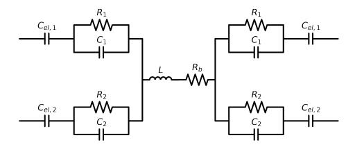
FIG. S6. Representation of the equivalent circuit used to fit the MD results.
