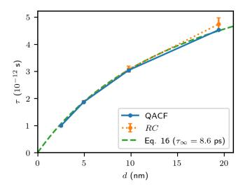
FIG. S10. Charge relaxation time as a function of the inter-electrode distance.  $\tau$  is estimated either as the integral of the normalized total charge ACF (blue solid line) or as the RC time (orange dotted line), using the total resistance at low frequency and the cell capacitance. The scaling of Eq. 16 is also shown (dashed green line).
