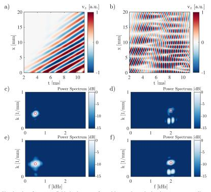
Figure S2. Simulated surface wave fields in the case of quasi-harmonic excitation in a two-part medium with shear moduli  $G_1 = 30$  kPa and  $G_2 = 60$  kPa and: a) h = 0.25 mm and f = 0.5 kHz, b) h = 1 mm and f = 2 kHz. Fourier kf power spectra of the wavefield (a) computed in part I (c) and part II (e) respectively; and Fourier kf power spectra of the wavefield (b) computed in part I (d) and part II (f) respectively.
