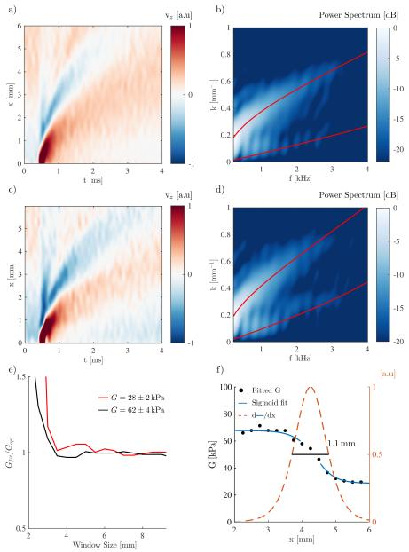
Figure 9. Space-time waveforms (XT plots) recorded experimentally across 6mm in a two-part phantom (see Fig.3) in (a) part I ( $G_1 = (28 \pm 2)$  kPa) and (c) part II ( $G_1 = (62 \pm 4)$  kPa) and their corresponding kf spectra (b) and (d), respectively. (e) Dependence of the reconstructed shear modulus on window size in each part of the phantom. (f) Dependence of mechanical modulus G on the distance from the A $\mu$ T source in the direction from part II to part I across the interface.
