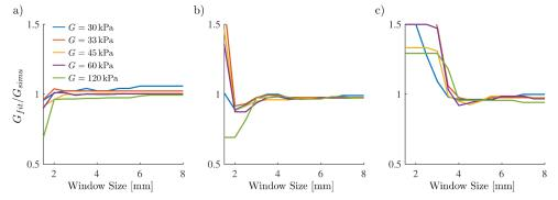
Figure 4. Window-size dependence of the reconstructed value of shear modulus G for different values of G shown in the insert to panel (a) at different layer thicknesses: (a) - h = 0.25 mm, (b) - h = 0.5 mm, (c) - h = 1 mm.
