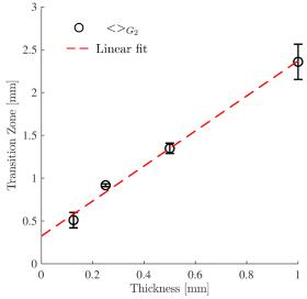
Figure 7. Dependence of the transition zone width on the thickness of a two-part medium. Shear modulus of the first part of the medium used in this figure is  $G_1 = 30$  kPa; in the second part shear moduli varied in the range of  $G_2 = (33-120)$  kPa. All depicted values correspond to mean values obtained for different values of  $G_2$ ; the error bars correspond to their variations. The straight line corresponds to fitting the points with a linear function (7)).
