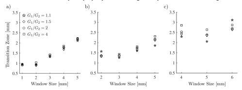
Figure 6. Dependence of the transition zone on window size at different layer thicknesses: (a) - h = 0.25 mm, (b) - h = 0.5 mm, (c) - h = 1 mm. Shear modulus of the first part of the medium used in this figure is  $G_1 = 30$  kPa. The ratio of moduli for the two parts is shown in the insert.
