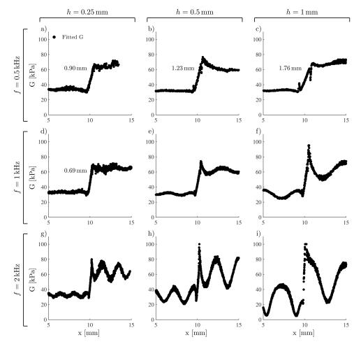
Figure S1. Dependence of the reconstructed shear modulus G on the distance from the source (black dots) in the twoparts medium with shear moduli  $G_1 = 30$  kPa and  $G_2 = 60$  kPa, respectively, for quasi-harmonic excitation. The excitation frequency and medium thickness are shown on the left and on the top of the panels, respectively. The lateral resolution in panel (e) though panel (i) is undetermined due to high fluctuations in the reconstructed moduli.
