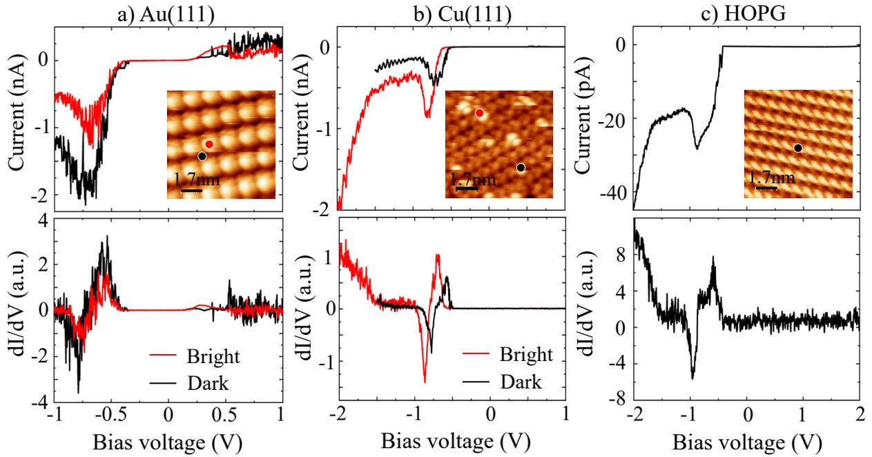
Figure 1: STS measurements on molecules in monolayer islands grown on a) Au(111), b) Cu(111), and c) HOPG substrates. For a) and b), the  $I - V$  and  $dI/dV$  curves have been acquired on molecules appearing either dark or bright at 0.3 V. The  $8.5 \times 8.5 \text{ nm}^2$  STM topographic images with the positions at which the spectra have been acquired are shown in the inset. a) 0.3 V, 50 pA, b) 0.3 V, 5 pA and c)  $-1.5 \text{ V}$ , 20 pA.
