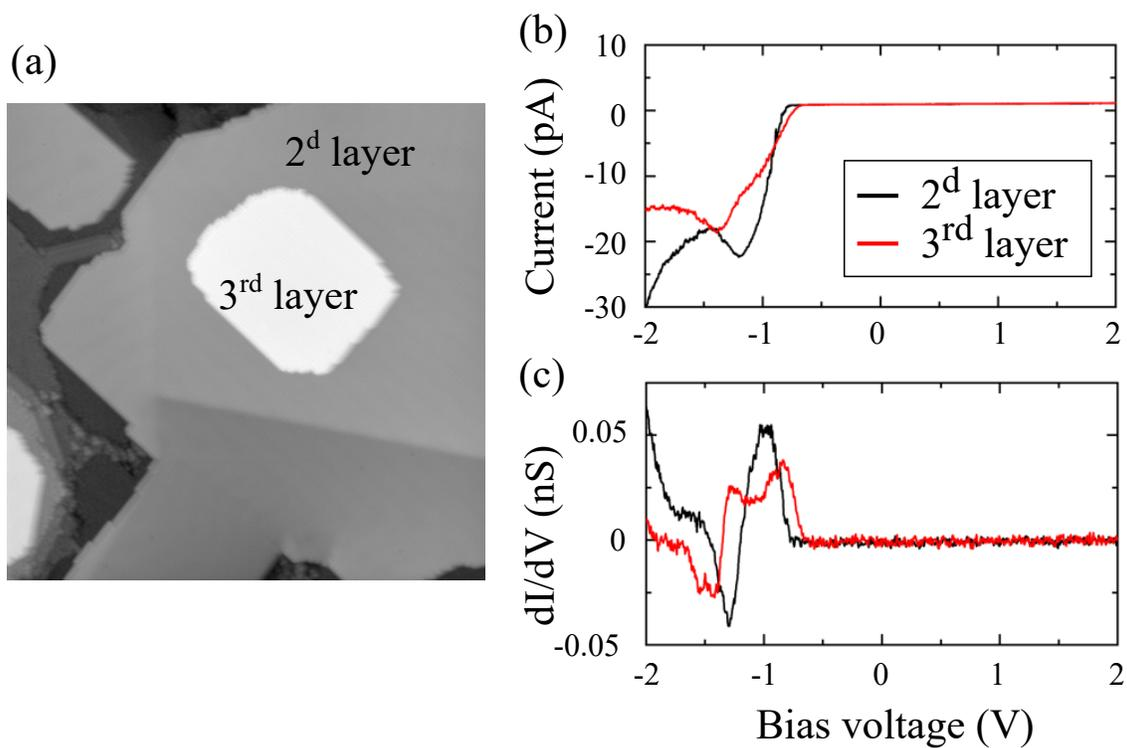
Figure 2: (a)  $150 \times 150 \text{ nm}^2$  topographic STM image of FeMPz island up to 3 ML high ( $-1.5 \text{ V}$ ,  $20 \text{ pA}$ ). (b) and (c)  $I-V$  and  $dI/dV$  curves recorded in constant current mode on the second (black curves) and the third layer (red curves). The presented curves are averaged over several molecules and measurements (2<sup>d</sup> layer: 20 curves on 4 molecules, 3<sup>rd</sup> layer: 15 curves on 3 molecules)
