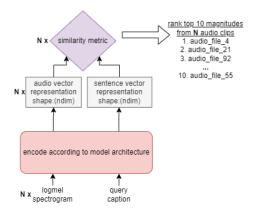
**Fig. 2**: Evaluation process: The logmel spectrogram of each audio clip in the evaluation set is encoded to obtain its corresponding vector representation. The query caption is likewise encoded to obtain the sentence vector representation. The similarity metric is then applied between each audio representation and the sentence representation to obtain a list of similarity values. These values are then ranked to obtain the relevance of each audio clip to the query caption.
