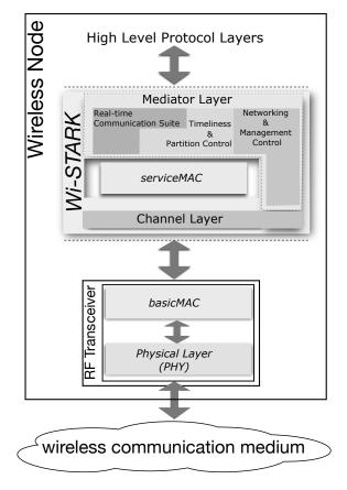
Figure 5 - The Wi-STARK Architecture
