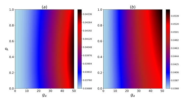
FIG. 5. Contour plots for the steady state heat flux,  $J_{ss}$  vs. system-HSE coupling,  $g_a$ , and coherence in the HSE, p. The couplings are (a)  $g_{12} = 50$ ,  $g_{23} = 25$ ,  $g_b = 10$  (b)  $g_{12} = 50$ ,  $g_{23} = 25$ ,  $g_b = 30$ .
