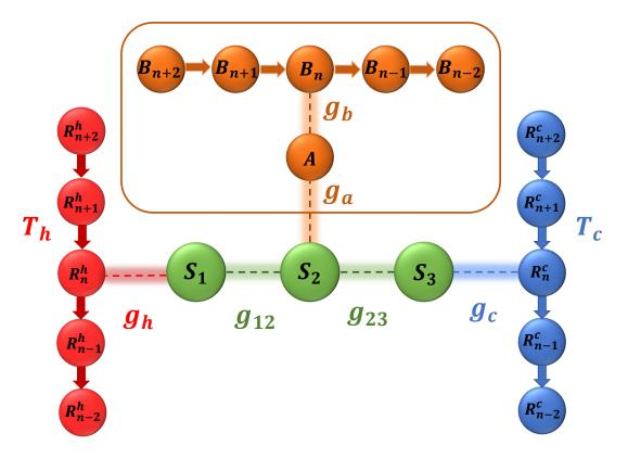
FIG. 1. A schematic representation of the model. The system qubits, denoted by  $S_1$ ,  $S_2$  and  $S_3$ , are interacting with each other and the qubits from the cold bath, hot bath and the hierarchical environment.
