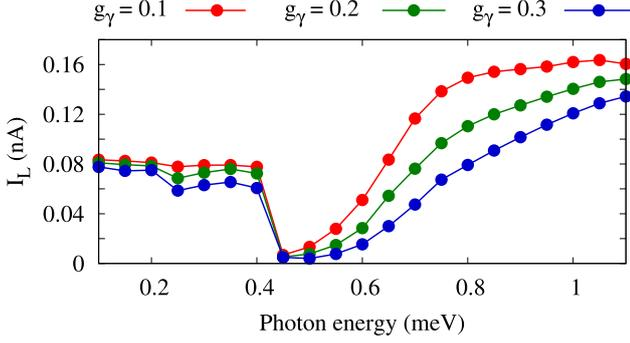
Figure 4: Total current from the left lead to the DQD system as a function of photon energy for  $g_\gamma = 0.1$  (red),  $0.2$  (green), and  $0.3$  meV (blue) in case of an  $x$ -polarized photon field. The initial photon number in the cavity is  $n_R = 1$ ,  $B = 0.1$  T,  $\kappa = 10^{-5}$  meV,  $V_g = 0.6$  meV and  $T_{L,R} = 0.5$  K.
