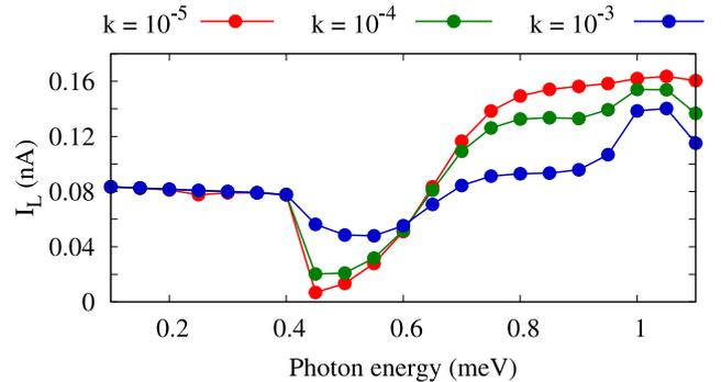
Figure 7: Total current from left lead to the DQD system as a function of photon energy for  $\kappa = 10^{-5}$  (red),  $10^{-4}$  (green), and  $10^{-3}$  meV (blue) in case of  $x$ -polarized photon field. The initial photon number in the cavity is  $n_R = 1$ ,  $B = 0.1$  T,  $g_\gamma = 0.1$  meV,  $V_g = 0.6$  meV and  $T_{L,R} = 0.5$  K.
