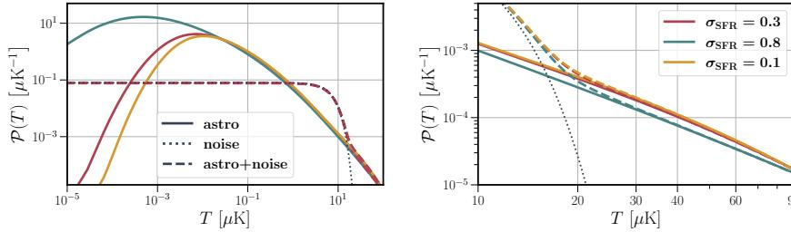
**Fig. 7** CO temperature PDF for the same cases as in Fig. 6. We show the PDF from the astrophysical contributions alone (solid), from the instrumental noise alone (dotted), and for their sum after mean subtraction (dashed); we assume  $\sigma_N = 5 \mu\text{K}$ . The right panel zooms in on the tail of the PDF, which in practice is the only range from which it is possible to extract astrophysical information.
