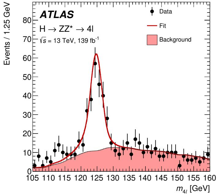
Figure 6: The  $m_{4\ell}$  data distribution from all subchannels combined (black points) is shown along with the signal-plus-background post-fit probability density function (red line). The  $p$ -value quantifying the agreement between the data and the fit model is 0.53.
