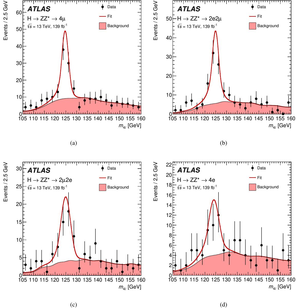
Figure 7: The  $m_{4\ell}$  data distribution (black points) for (a)  $4\mu$ , (b)  $2e2\mu$ , (c)  $2\mu2e$ , and (d)  $4e$  events is shown along with the signal-plus-background post-fit probability density function (red line). The  $p$ -values quantifying the agreement between the data and the fit model are (a) 0.92, (b) 0.10, (c) 0.83, and (d) 0.97.
