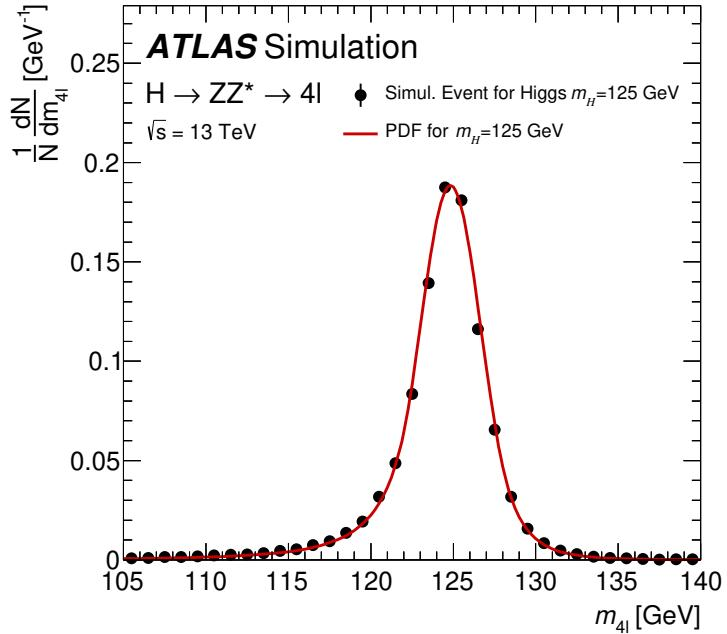
Figure 5: The probability density function derived from signal MC simulation using the per-event resolution (red line) is shown in comparison with the  $m_{4\ell}$  distribution in signal MC simulation (black points) for  $m_H = 125 \text{ GeV}$ . The probability density function is derived for each channel separately and they are added together assuming predicted yields. Both the probability density function and the MC simulation are normalised to unity.
