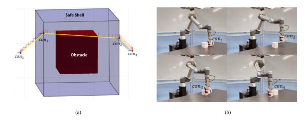
Figure. 8 Motion plans for the transferring task. (a) The motion plan in SE(3). (b) Execution the motion plan in  $\mathcal{J}$ .
