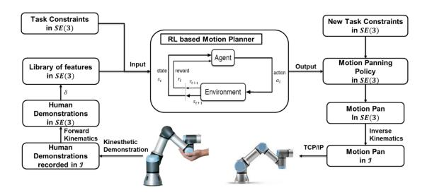
Figure. 4 Framework of the RL based user-guided motion planning.
