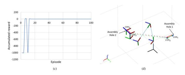
**Figure. 10** Generate motion plans for the assembling task after the feature of a new human demonstration is added to the library. (a) Critical configurations and the motion plan in  $\mathcal{J}$  for the assembling task after an additional human demonstration is provided. (b) Additional human demonstration for picking up a span. (c) The training process of the assembling task after the feature of a new human demonstration is added. (d) Motion plan in *SE*(3).
