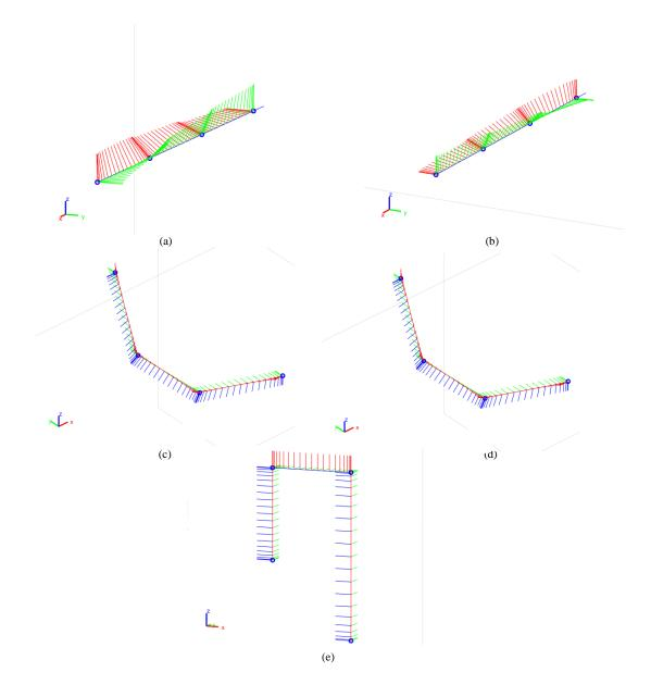
Figure. 6 Human demonstrations in SE(3). (a) Screwing task 1. (b) Screwing task 2. (c) Pouring task. (d) Filling task. (e) Stacking task. Using forward kinematics, corresponding configurations of end-effector in SE(3) are shown in Fig. 6. Using Eqn. (14), features of human demonstrations are saved as  $LB = \{HD_1, HD_2, ..., HD_5\}$  in the library shown in Table 5.
