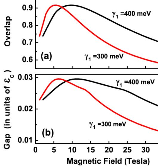
FIG. 7 Panel (a): Overlap of the ground state wave function of  $\nu = 1/2$  state with the Pfaffian state as a function of the magnetic field. Panel (b): the collective excitation gap of the  $\nu = 1/2$  state as a function of the magnetic field. The data are shown for the Landau level  $0_{-1}^{(+)}$  of the bilayer graphene and for two values of the interlayer hopping integral,  $\gamma_1$ . Reproduced with permission from (Apalkov and Chakraborty, 2011).
