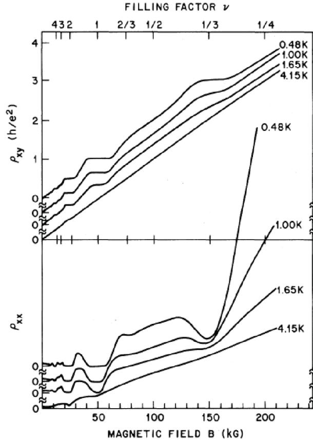
FIG. 1 Non-diagonal and diagonal resistivities,  $\rho_{xy}$  and  $\rho_{xx}$ , as a function of magnetic field,  $B$ . The sample is GaAs- $\text{Al}_{0.3}\text{Ga}_{0.7}\text{As}$  with electron density of  $n = 1.23 \times 10^{11} \text{ cm}^{-2}$  and mobility  $\mu = 90000 \text{ cm}^2/\text{Vs}$  (Adapted from (Tsui et al., 1982)).
