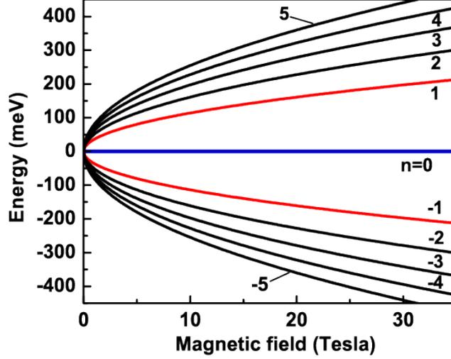
FIG. 4 The first few Landau levels of graphene monolayer as a function of perpendicular magnetic field. The Landau levels are labeled with integer index  $n$ , where positive and negative  $n$  correspond to the conduction and valence bands, respectively. The red and blue lines mark the Landau levels for which the QHE can be observed.
