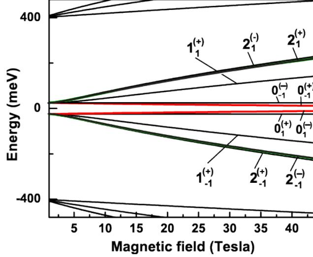
FIG. 6 A few lowest Landau levels of bilayer graphene as a function of the magnetic field. The bilayer graphene has the AB stacking. The Landau levels of both  $K$  and  $K'$  are shown. The red lines show special Landau levels, at which the  $\nu = 1/2$  Pfaffian incompressible state can be realized. The bias voltage is 5 meV and interlayer hopping integral is  $\gamma_1 = 400$  meV.
