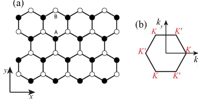
FIG. 3 (a) Honeycomb crystal structure of graphene monolayer. Two equivalent sublattices A and B are marked by open and filled dots. (b) The first Brillouin zone of monolayer graphene. Two valley  $K$  and  $K'$  are also shown.
