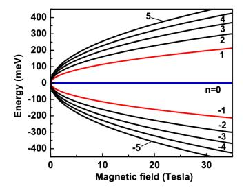
FIG. 4 The first few Landau levels of graphene monolyaer as a function of perpendicular magnetic field. The Landau levels are labeled with integer index n, where positive and negative n correspond to the conduction and valence bands, respectively. The red and blue lines mark the Landau levels for which the FQHE can be observed.
