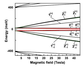
FIG. 6 A few lowest Landau levels of bilayer graphene as a function of the magnetic field. The bilayer graphene has the AB staking. The Landau levels of both K and K' are shown. The red lines show special Landau levels, at which the  $\nu=1/2$  Pfaffian incompressible state can be realized. The bias voltage is 5 meV and interlayer hopping integral is  $\gamma_1=400$  meV.
