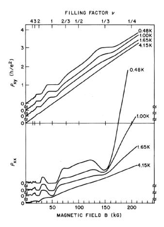
FIG. 1 Non-diagonal and diagonal resistivities,  $\rho_{xy}$  and  $\rho_{xx}$ , as a function of magnetic field, B. The sample is GaAs-Al<sub>0.3</sub>Ga<sub>0</sub>.7As with electron density of  $n=1.23\times10^{11}~{\rm cm}^{-2}$  and mobility  $\mu=90000~{\rm cm}^2/{\rm Vs}$  (Adapted from (Tsui et al., 1982)).
