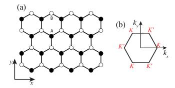
FIG. 3 (a) Honeycomb crystal structure of graphene monolayer. Two equivalent sublattices A and B are marked by open and filled dots. (b) The first Brillouin zone of monolayer graphene. Two valley K and K' are also shown.
