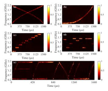
Fig. 3. Measured time-frequency diagrams by the proposed STFT scheme for (a) dual-chirp LFM signal, (b) non-linearly frequency-modulated signal, (c) step-frequency signal, (d) frequency-hopping signal, (e) a specially designed signal whose time-frequency characteristic is the abbreviation "ECNU" of "East China Normal University".
