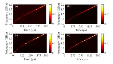
Fig. 2. Measured time-frequency diagrams of the LFM signals with a bandwidth ranging from 0.2 GHz to 2.2 GHz and a time duration of 500  $\mu$ s and 1500  $\mu$ s. The frequency of the triangular wave is (a) and (b) 100 kHz, (c) and (d) 50 kHz.
