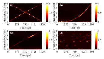
Fig. 5. Measured time-frequency diagrams by the proposed STFT scheme for (a) dual-chirp LFM signal, (b) non-linearly frequency-modulated signal, (c) step-frequency signal, (d) frequency-hopping signal, with a bandwidth ranging from 0 to 4 GHz.
