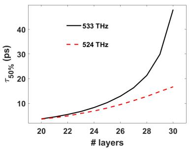
**Figure 5.** Delay time of the transmitted light pulses through the  $(PVK/CA)_{NL}$ /diarylethene1/(CA/PVK)\_{NL} microcavity, corresponding to 50% of the intensity of the initial signal, as a function of the number of layers NL (black solid curve is related to diarylethene1 in the open form, red dashed curve is related to diarylethene1 in the closed form).
