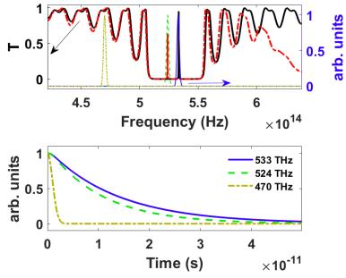
**Figure 4.** (above) Transmission spectra of the microcavity (PVK/CA)<sub>25</sub>/diarylethene1/(CA/PVK)<sub>25</sub>, with diarylethene1 in the open form (solid black curve) and in the closed form (dashed red curve), and spectral shapes of three light pulses centred at 470, 524 and 533 THz. (below) Time-resolved transmitted signals through the microcavity.
