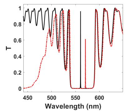
**Figure 3.** Transmission spectra of the microcavity (PVK/CA)<sub>25</sub>/diarylethene1/(PS/PVK)<sub>25</sub> with diarylethene1 in the open form (solid black curve) and in the closed form (dashed red curve).
