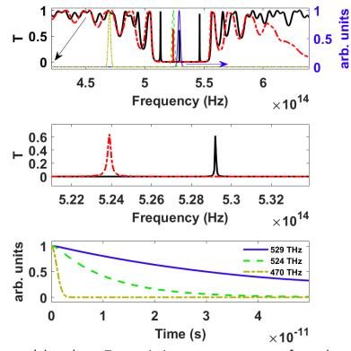
**Figure 6.** (above) Transmission spectra of the microcavity (PVK/CA)<sub>NL</sub>/(randomPVK/PS)/diarylethene1/(randomPVK/PS)/(CA/PVK)<sub>NL</sub>, with diarylethene1 in the open form (solid black curve) and in the closed form (dashed red curve), and spectral shapes of three light pulses centred at 470, 524 and 529 THz. (middle) Magnification of the transmission spectrum in the region of the central cavity modes. (below) Time-resolved transmitted signals through the microcavity.
