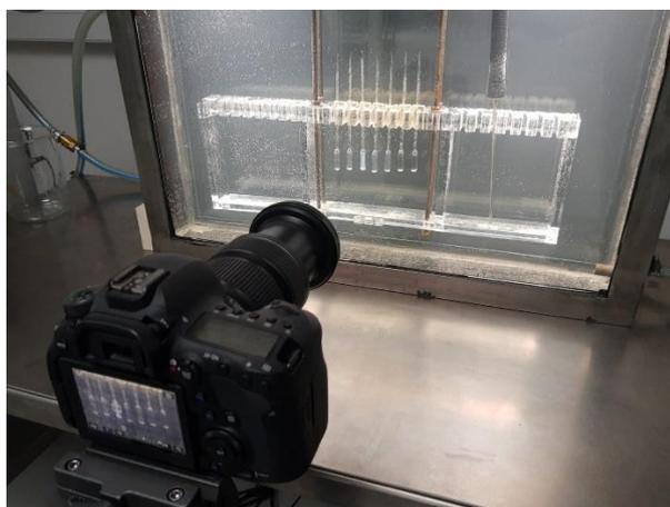
**Figure 1** The basic part of the innovative system for determining phase equilibria via the automatized photo-observation of menisci between coexisting liquid phases in mixtures of limited miscibility.
