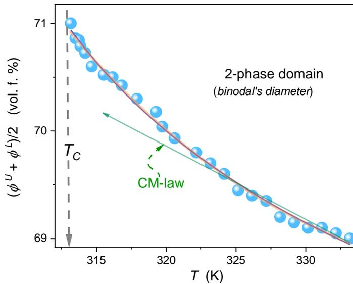
**Figure 7** The focused presentation of 3-picoline – D<sub>2</sub>O binodal curve diameter, given in Fig. 4. The curves are related to Eq. 4a, with exponents  $\beta = 0.325$ , and  $\alpha = 0.12$  (red curve) and Eq. 4b, where ' $2\beta$ ' anomaly is introduced (grey curve, slightly broadened). Both curves overlap. The green line terminated by the arrow shows the hypothetical Cailletet – Mathias law of rectilinear diameter [19-21], illustrating its essential inadequacy.
