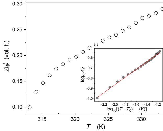
**Figure 5** Changes of the order parameter in 3-picoline – deuterium oxide mixture of limited miscibility. The inset shows the test via Eq. (8), yielding the exponent  $\beta_{eff.} = 0.365 \pm 0.02$  using the log-log-scale with the adjustable critical temperature.
