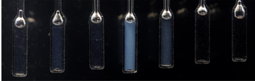
**Figure 2** The photo of 3-picoline – deuterium oxide mixtures in the surrounding of the critical concentration, near the critical temperature. The white-bluish critical opalescence, signaling the vicinity of the critical point, is visible.
