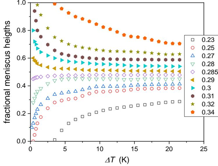
**Figure 3** The temperature evolution of fractional meniscus heights (f.m.h.,  $h$ ) for coexisting phases in 3-picoline –  $D_2O$  mixtures.
