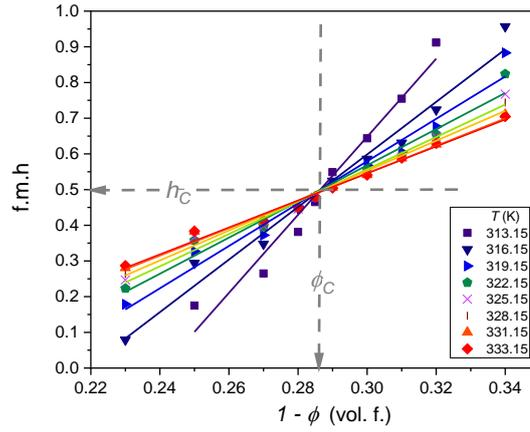
**Figure 8** Isothermal behavior of fractional meniscus height (f.m.h.) for different 3-picoline – D<sub>2</sub>O mixtures: the values of selected temperatures are given in the plot. The linear behavior validates the description via Eq. (10). The intersection of lines yields the critical concentration ( $\phi_c$ ) and the coupled critical value of f.m.h. ( $h_c$ ). The plot is for data given in Fig. 3.
