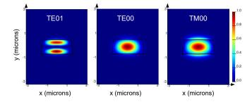
FIG. 2. Electric field profiles for a CdS core and  $SiO_2$  cladding, at 1550 nm for the TE01 mode and at 3100 nm for the TE00 and TM00 modes.
