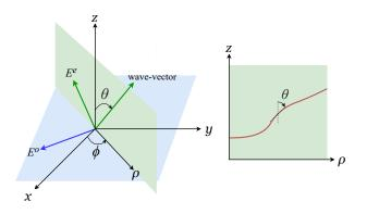
FIG. 1. Propagation geometry. We assume the path of the waveguide lies in the green plane. This plane is uniquely specified by the fact that it contains the z axis and makes an angle  $\phi$  with the x axis.
