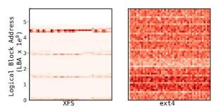
Figure 4 LBA heatmap over time during enumeration.
