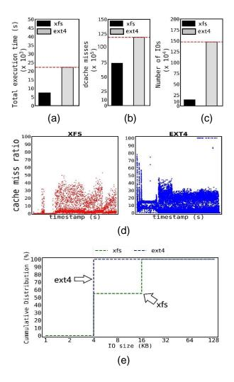
Figure 3 Object Store services Management Workload: Lexicographic Enumeration (a) total execution time; (b) dcache misses per server; (c) number of IOs incurred; (d) page cache miss ratio; (e) Cummulative Distribution (CDF) IO block-size (KB) for xfs and ext4.
