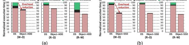
Figure 6 Normalized latency breakdown for user-applications comparing conventional OS-based with Object-Drive OSD with (a) HDD; and (b) SSD, storage media backend. IO type: Object Data (OD), Object Metadata (OM) and Filesystem Metadata (FSM).
