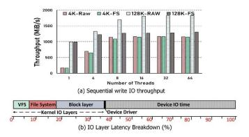
Figure 2 Impact of IO-layers: (a) Sequential write IO (fio) throughput on block NVMe device with (FS) and without (RAW) file-system.; (b) Normalized time-spent by an IO request in an IO-layer.
