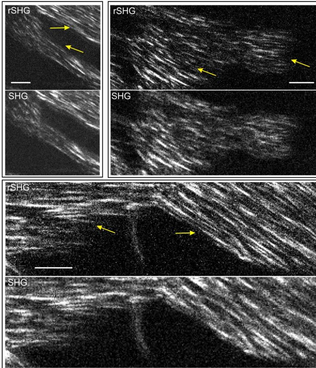
**Fig. 2.** Resolution advantage of rSHG vs. SHG on rat-tail collagenous tissues at different levels of detail. Yellow arrows point to sample areas where rSHG's resolving power is well visible. Scale bars: 3 $\mu$ m.
