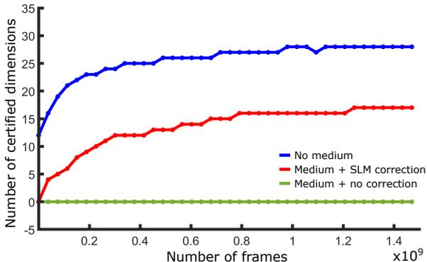
Figure 4. **Certified dimension analysis.** Number of certified dimensions for different total number of frames without medium (blue curve), with medium and SLM correction (red curve), with medium and no correction (green curve).
