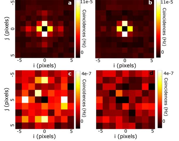
Figure 6. **Conditional probability images before and after cross-talk removal.** (a)  $\Gamma_{ijkl}^{(raw)}$  and (b)  $\Gamma_{ijkl}$  acquired in the position basis configuration without medium. The reference pixel  $(k, l)$  is the central pixel  $(0, 0)$ . (c)  $\Gamma_{ijkl}^{(raw)}$  and (d)  $\Gamma_{ijkl}$  acquired in the position momentum basis configuration without medium. The reference pixel  $(k, l)$  is the central pixel  $(0, 0)$ .  $7 \times 10^8$  frames were acquired.
