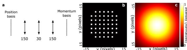
Figure 8. **Measure of unbiasedness.** **a.** Experimental configuration representing the optical transformation that links the position and momentum bases in our experiment. **b.** Spatial arrangement of the 45 selected pixels in the position and momentum optical planes. **c.** Sinc-shaped intensity distribution produced by a pixel located in one optical plane into the reciprocal optical plane.
