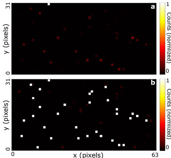
Figure 7. **Hot pixels identification.** (a) Intensity image obtained by summing  $1.2 \times 10^9$  frames acquired with no light on the sensor. (b) Same image with the 32 identified hot pixels appearing in white.
