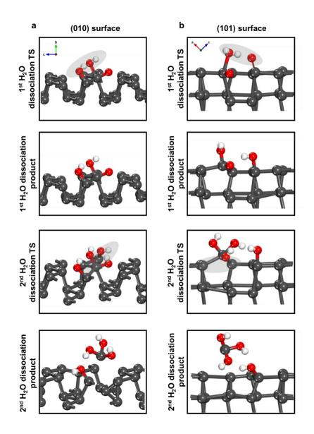
**Figure 4.** DFT-optimized transition and product state structures for dissociation of the  $1^{st}$  and  $2^{nd}$  H<sub>2</sub>O molecule at the oxidized (a) (010) and (b) (101) b-As surfaces resulting in volatilization of As atom as As(OH)<sub>3</sub> molecule. The highlighted grey regions corresponds to bond making and breaking in the transition structures. In these structures, As atoms are in dark grey color, O in red, and H in white.
