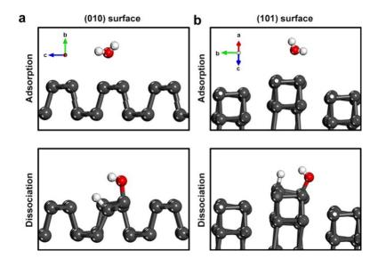
**Figure 2.** DFT-optimized structures for the adsorption (top) and dissociation (bottom) of  $H_2O$  on (a) (010) and (b) (101) surfaces of b-As. In these structures, As atoms are in dark grey color, O in red, and H in white. The adsorption energies and interatomic distances for these structures are reported in Table 1.
