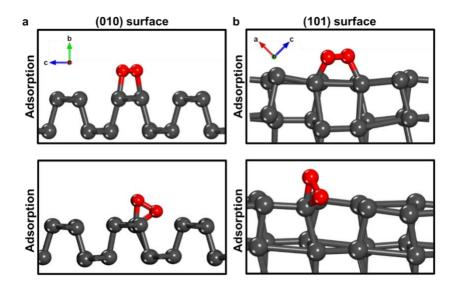
**Figure S3:** DFT-optimized structures for the other modes of O<sub>2</sub> adsorption: di- $\sigma$  adsorption (top) and  $\pi$ -adsorption (bottom) on (a) (010) and (b) (101) b-As surface. In these structures, As atoms are in dark grey and O in red.
