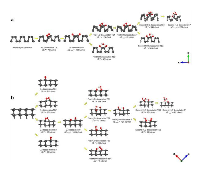
**Figure S5.** Flow diagram depicting the possible mechanistic routes involved in the sequential dissociation of oxygen followed by the dissociation of two water molecules with the corresponding reaction barriers and energies over the (a) (010) and (b) (101) b-As surface. In these structures, As atoms are in dark grey, O in red, and H in white.
