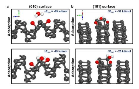
**Figure S9.** DFT-optimized two different conformational structures (top and bottom) for molecular adsorption of the water molecule over the two oxidized As atoms present on the (a) (010) and (b) (101) b-As surface with As vacancy. In these structures, As atoms are in dark grey, O in red, and H in white.
