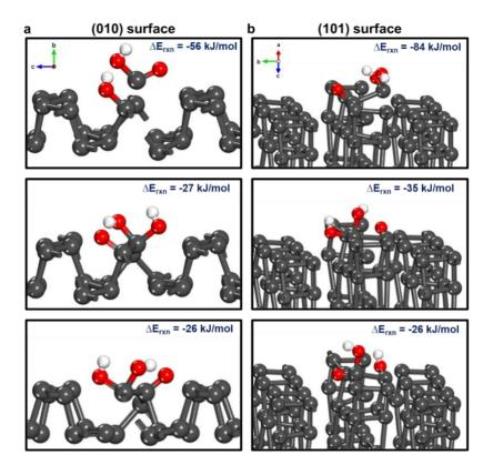
**Figure S10.** DFT-optimized structures of the other possible higher energy configurations for dissociation of the first water molecule over the oxidized (a) (010) and (b) (101) b-As surface with a As vacancy. In these structures, As atoms are in dark grey, O in red, and H in white.
