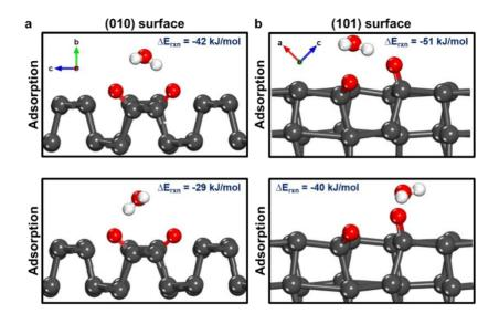
**Figure S4:** DFT-optimized conformational structures (top and bottom) for molecular adsorption of the water molecule over the two oxidized As atoms present on the (a) (010) and (b) (101) b-As surfaces. Low coverages of  $1/4^{\text{th}}$  of a surface on the (010) surface and  $1/8^{\text{th}}$  of a surface on the (101) surface were considered. In these structures, As atoms are in dark grey, O in red, and H in white.
