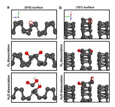
**Figure 5:** DFT-optimized structures for the (010) and (101) b-As surfaces showing a vacancy on the surface (top, the missing site is highlighted with a red dotted circle), dissociation of  $O_2$  (center) and the first water molecule (bottom) at the As sites adjacent to the vacancy on the (a) (010) and (b) (101) b-As surfaces resulting in volatilization of an As atom as AsO(OH) molecule. In these structures, As atoms are in dark grey color, O in red, and H in white.
