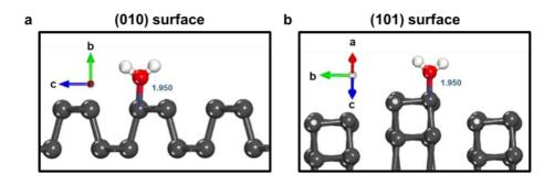
**Figure S2.** The initial structures of water adsorption over the bare (a) (010) and (b) (101) surfaces of b-As. In both cases the As-O distance was kept at 1.95 Å corresponding to low coverages of  $1/8^{\text{th}}$  of a surface on the (010) surface and  $1/16^{\text{th}}$  of a surface on the (101) surface. In these structures, As atoms are in dark grey, O in red, and H in white.
