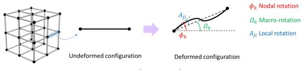
Figure 1. Physical meanings of nodal rotation  $\phi_k (= \Omega_k - e_{ijk}A_{ij})$ , macro-rotation  $\Omega_k$ , and local rotation  $A_{ji}$ .
