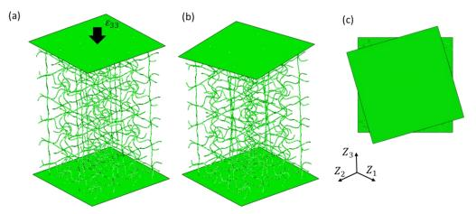
Figure 7. Axial-twisting (AT) coupling of 422 lattice: (a) initial geometry, (b) deformed shape, (c) top view of deformed shape.
