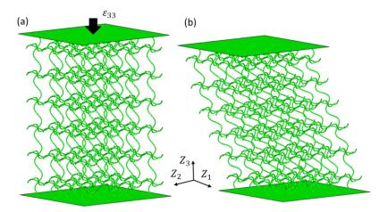
Figure 4. Axial–shear (AS) coupling of  $\overline{1}$  lattice: (a) initial geometry and (b) deformed shape.
