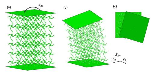
Figure 5. Bending–twisting (BT) coupling of  $\overline{1}$  lattice: (a) initial geometry, (b) deformed shape, and (c) top view of deformed shape.
