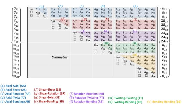
Figure 2. Mechanical couplings in the decoupled micropolar elasticity tensor q.
