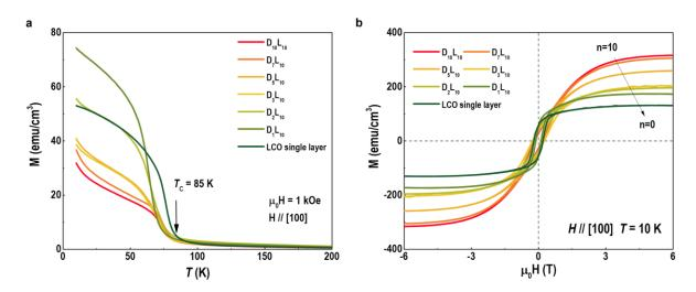
**Figure S4. Magnetization characterizations of D**<sub>n</sub>L<sub>10</sub> **SLs.** (a) *M*-*T* curves of D<sub>n</sub>L<sub>10</sub> SLs for  $1 \le n \le 10$ . The *M*-*T* curves were measured under a magnetic field of 1 kOe applied along the [100] orientation after field-cooling. *M*-*T* results show that LCO single layer and all SLs exhibit clear paramagnetic-ferromagnetic phase transitions. *T*<sub>C</sub> of LCO single layer is ~ 85 K,
