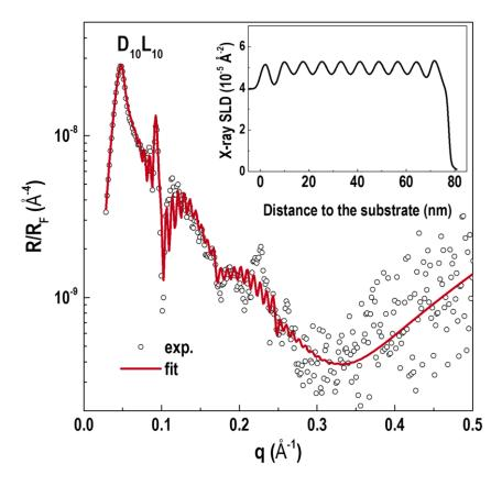
**Figure S5. XRR of D**<sub>10</sub>L<sub>10</sub> **SL.** The solid line is the best fit to the experimental data (open symbols). The thicknesses of DSO and LCO layers are  $39.2 \pm 4.6$  Å and  $38.5 \pm 3.9$  Å, respectively. The DSO/LCO bilayer repeats 10 times. The total thickness of D<sub>10</sub>L<sub>10</sub> SL is 79.8  $\pm$  0.9 nm. Inset shows the X-ray scattering length density (SLD) profile of D<sub>10</sub>L<sub>10</sub> SL. The X-
