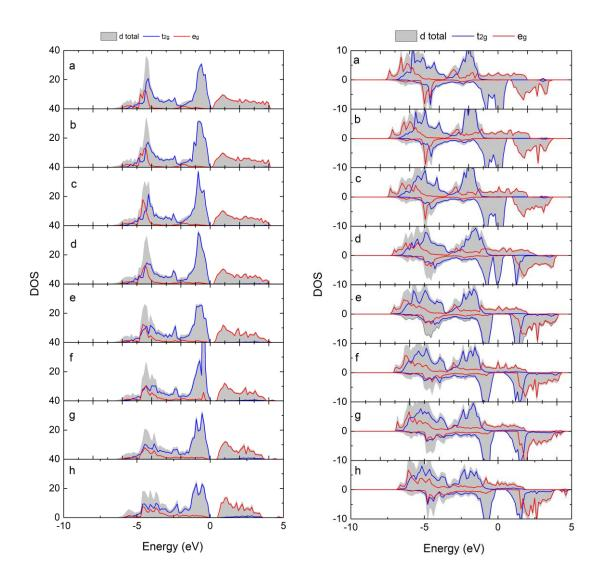
Figure S11. Projected density of states (DOS) for LS (lefthand) and IS (righthand) states LaCoO<sub>3</sub> with rotation amplitude varying from 0% to 7%. The gray area, bule lines, and red lines represent the Co ions d total,  $t_{2g}$  and  $e_{g}$ , respectively.
