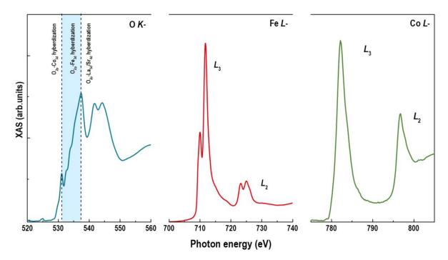
**Figure S8. XAS measurements of**  $F_1L_1$  **SL**. XAS at O *K*-, Fe *L*-, and Co *L*-edges were measured at room temperature. XAS results indicate that Fe ions and Co ions keep +3, indicating the negligible charge transfer between Co and Fe ions. This fact is important for analyzing the spin states of Co ions within  $F_1L_1$  SL.
