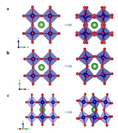
**Figure S10. Crystal structures with different tilting patterns.** (a), (b), and (c) Schematic crystal structures of  $2 \times 2 \times 2$  supercells along the pseudocubic [100], [001], and [110] zone axis, respectively. The supercells are without (lefthand) and with (righthand) octahedral tilt, corresponding to the  $a^0a^0a^0$  non-tilted pattern (S<sub>1</sub>L<sub>1</sub> SL) and  $a^-a^-c^+$  tilt pattern (D<sub>1</sub>S<sub>1</sub> and F<sub>1</sub>L<sub>1</sub> SLs), respectively.
