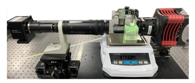
Figure 2: Image of experimental setup. A green light laser (540nm) is used to create coherent light, which first passes through a collimating lens, then through a linear polarizer (0°) and quarter waveplate (45°) to create left-handed circular polarized light. The light is incident upon the gelatin cuboid and emerges with an accumulated phase retardation  $\Delta$  and orientation  $\psi$  and is then recorded by a Photron Crysta PI-5WP high-speed polarization camera.
