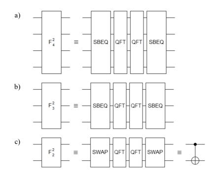
FIG. 2. Second-degree QFG for a) 4 qubits, b) 3 qubits, and c) 2 qubits, where SBEQ = SWAP gate.
