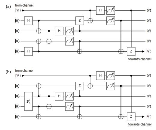
FIG. 25. Quantum repeaters based on entanglement swapping: a) the original version<sup>30</sup>, and b) based on a  $F_2^{I}$  gate that generates two parallel and independent Bell states  $|\beta_{00}\rangle$ .
