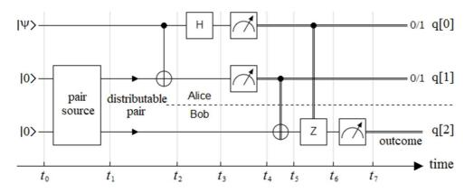
FIG. 14. Quantum teleportation protocol, where the pair-source module can emit maximally, non-maximally, and rough entangled states. The protocol starts from the side of Alice (sender) who emits the pair of particles with some of the three types of entanglement, keeping one particle and sending the other to Bob (receiver).
