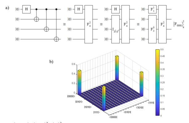
FIG. 8.  $|GHZ_4\rangle \equiv |F_{0000}\rangle_4^2 = |F\rangle_4^2$  state, where a) represents equivalences between gates, while, b) shows a 3D implementation of its density matrix.
