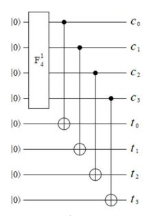
FIG. 20. Entanglement parallelization: Based on a  $F_4^1$  gate, each output pair  $\{c_i, t_i\}$   $(\forall i \in [0,3])$  shares a state  $|\beta_{00}\rangle$  among them, but they are completely uncorrelated with the members of the other pairs.
