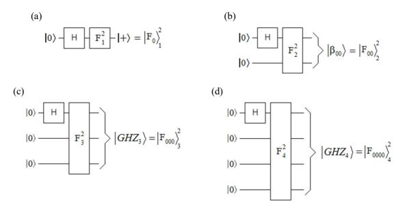
FIG. 18. Quantum stretching: a) for a single qubit, the state  $|+\rangle = |F_0\rangle_1^2$  is obtained with  $F_1^2 = I_{2^l \times 2^l}$ , b) for two qubits, the output is  $|\beta_{00}\rangle = |F_{00}\rangle_2^2$ , c) for three qubits, we have  $|GHZ_3\rangle = |F_{000}\rangle_3^2$ , and for four qubits, the output is  $|GHZ_4\rangle = |F_{0000}\rangle_4^2$ .
