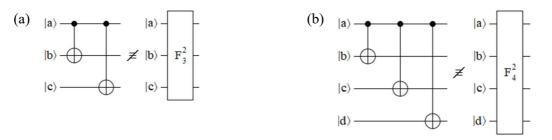
FIG. 12. Equivalences that do not hold between gates according to different combinations of the CBS inputs: a)  $|a\rangle$ ,  $|b\rangle$  and  $|c\rangle$  for 3 qubits, and b)  $|a\rangle$ ,  $|b\rangle$ ,  $|c\rangle$ , and  $|d\rangle$  for 4 qubits.
