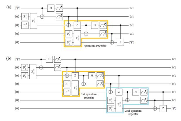
FIG. 26. Quantum repeaters based on teleportation cascade: a) only one quantum repeater and b) two quantum repeaters in consecutive teleportations configuration.
