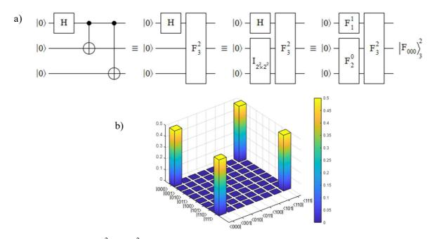
FIG. 7.  $|GHZ_3\rangle \equiv |F_{000}\rangle_3^2 = |F\rangle_3^2$  state, where a) represents equivalences between gates, while, b) shows a 3D implementation of its density matrix.
