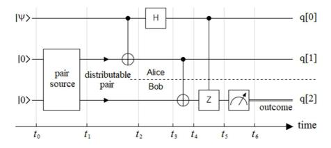
FIG. 16. A simplified version of the quantum teleportation protocol without quantum measurement modules in qubits q[0], and q[1], allows the implementation of this protocol in any physical machine of IBM  $Q^{18}$ , for example in one of the 5-qubits like Lima.
