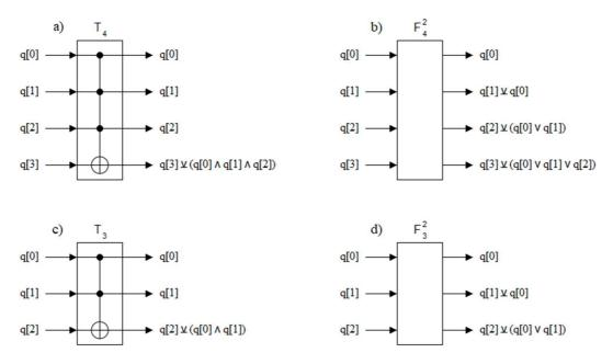
FIG. 3. Toffoli vs QFG of second degree: a) Toffoli of 4 qubits, b) QFG of 4 qubits, c) Toffoli of 3 qubits, and QFG of 3 qubits.
