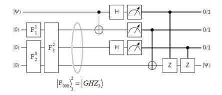
FIG. 23. Quantum secret sharing is based on an entangled source of three particles ( $|GHZ_3\rangle$ ) which is implemented based on quantum Fourier gates like those of Fig. 7(a).
