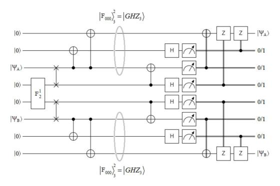
FIG. 24. Parallel quantum secret sharing is based on two independent sources of  $|GHZ_3\rangle$  states, for the simultaneous transmission of two different states,  $|\psi_A\rangle$  and  $|\psi_B\rangle$ , thanks to a configuration that uses only one  $F_2^I$  gate.
