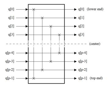
FIG. 1. Swapping-between-equidistant-qubits (SBEQ) gate for p qubits are exchanged. Individual exchanges occur between qubits opposite by the center, in the correct order from the ends towards the center, both for odd and even p.
