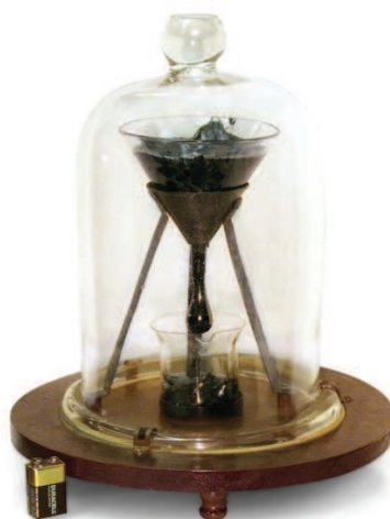
Fig. 1. The University of Queensland pitch drop experiment, demonstrating the viscosity of bitumen. 13
