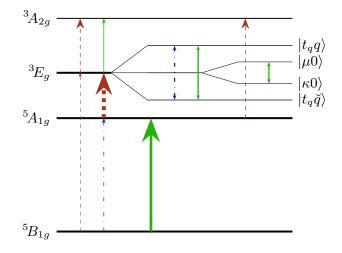
FIG. 6. Sketch of the transitions allowed by intersite hopping induced by light (green solid lines), spin-orbit coupling (brown dashed lines) and Jahn-Teller orthorhombic distortions (blue dashed-dotted lines). Thicker arrows indicate stronger interactions, corresponding to transitions between  ${}^{5}B_{1g}$  and  ${}^{5}A_{1g}$  mediated by intersite hopping and between  ${}^{5}A_{1g}$  and  ${}^{3}E_{g}$  mediated by spin-orbit coupling.
