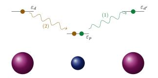
FIG. 3. Diagram of the electron transfer between neighbouring sites mediated by oxygen ions, induced by the interaction with an electromagnetic field. In the process, there is a first transition from oxygen p-orbital to neighbouring manganese d'-orbital. A second transition involves a transfer from a manganese d-orbital to an oxygen p-orbital.
