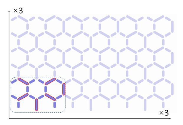
Figure S1 | Sample design of Kagome ASI. The dashed box in the bottom left is the basic repeating unit of the sample design. The  $\alpha$  magnets with adjustable length are highlighted with red boundaries.
