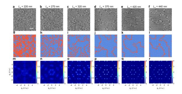
Figure S3 | Experimental results of spin/moment configurations for all six measured samples. a-f, MFM images. Scale bar, 2  $\mu$ m. g-h, spin configurations and vertex distributions extracted from (a-f). Type K-I and K-II vertices are shown in blue and red, respectively. m-r, corresponding maps of magnetic structure factors calculated respectively from the spin configurations in (g-h).
