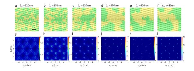
Figure S6 | Experimental results of magnetic charge configurations for all six measured samples. a-f, magnetic charge distributions corresponding to MFM images in Figs. S3a-S3f, respectively. Green and yellow denote two phases of magnetic charge ordering. g-l, maps of magnetic charge structure factors associated with (a-f).
