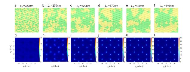
Figure S7 | Monte Carlo simulation results of magnetic charge. a-d, magnetic charge distributions. Green and yellow denote two phases of magnetic charge ordering. g-l, maps of magnetic charge structure factors associated with (a-f).
