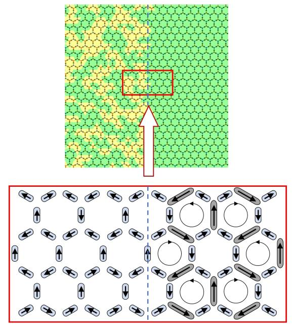
Figure S9 | **Kagome ASI with composite ground state.** The top figure shows spin and charge configurations of the ground state with spin liquid and spin crystal on left and right sides in the same Kagome lattice. Green and yellow colors denote two phases of magnetic charge. The bottom figure is an expanded view of the arrangement of nanomagnets within the red frame of the top figure.
