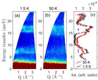
**Figure 8.** Inelastic neutron scattering data obtained with incident energy  $E_i = 25$  meV at two temperatures (a) 1.5 K and (c) 50 K. (c)  $|\mathbf{Q}|$ -integrated cuts ( $|\mathbf{Q}| = [1 - 2.5] \text{ Å}^{-1}$ ) of inelastic scattering showing the presence of two bands of crystal field excitations. Vertical blue lines in (c) indicate the instrumental energy resolution (full width at half-maximum).
