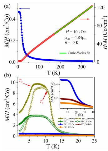
**Figure 3.** Magnetic susceptibility,  $\chi$ , and inverse magnetic susceptibility,  $1/\chi$ , as a function of temperature, *T*, measured using ground single crystal sample of NaCo<sub>2</sub>(SeO<sub>3</sub>)<sub>2</sub>(OH) measured at 10 kOe. (b) Magnetization curves of NaCo<sub>2</sub>(SeO<sub>3</sub>)<sub>2</sub>(OH) measured in different magnetic fields (*H* = 100 Oe - 50 kOe) below 25 K.
