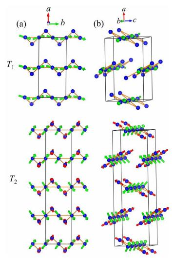
**Figure 7.** The proposed magnetic models for the two magnetic transitions, 11 K ( $T_1$ ) and 6 K ( $T_2$ ) are visualized in two different crystallographic orientations. The magnetic structure at 11 K is described within the same unit cell as the nuclear structure, whereas the structure at 6 K is doubled along the *a*-axis (i.e. 2*a*, *b*, *c*).
