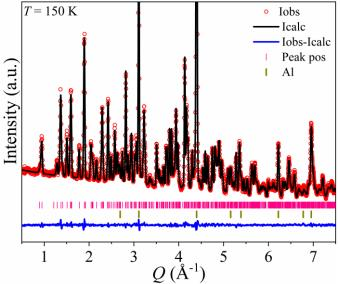
**Figure 1.** The Rietveld profile fit of the neutron powder diffraction data collected on HB2A using  $\lambda = 1.54$  Å at 150 K. The refinement was performed using a structural model with orthorhombic symmetry in the *Pnma* (no.62) space group. No evidence of any impurity phases was detected within the instrument sensitivity. The refined parameters are  $R_{wp}(\%) = 2.26$ , a = 13.2299(2) Å, b = 6.02287(9) Å, c = 8.32157(3) Å.
