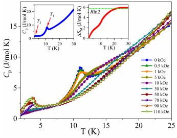
**Figure 5.** The specific heat curves of NaCo<sub>2</sub>(SeO<sub>3</sub>)<sub>2</sub>(OH) obtained for applied magnetic fields in 0 - 110 kOe range. A significant influence of the external magnetic field on both  $T_1$  and  $T_2$  transitions is observed. The insets show a zoomed view of the two magnetic transitions measured at H = 0 T, and the evaluated magnetic entropy of NaCo<sub>2</sub>(SeO<sub>3</sub>)<sub>2</sub>(OH), respectively.
