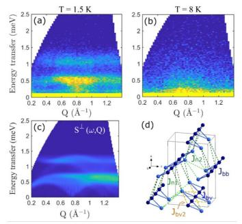
**Figure 9.** (a) Spin-wave excitation spectrum of measured at 1.5 K using  $E_i = 3.8 \text{ meV}$ . (b) Inelastic spectrum measured in the partial ordered state at 8 K,  $(T_1 < T < T_2)$  (c) Calculated spin-wave spectrum using a simple Heisenberg Hamiltonian model that includes three intra-chain ( $J_{bv}$ ,  $J_{bb}$ ,  $J_{bv2}$ ) and two interchain ( $J_{n1}$ ,  $J_{n2}$ ) exchange interactions. The magnetic exchange pathways are shown in (d).
