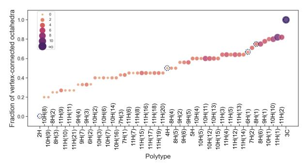
Figure 4. The intermediate close-packed polytypes between cubic perovskite (3C) and delta phase (2H) of APbX<sub>3</sub> with 4-11 close-packed layers with different fraction of vertex-connected PbI<sub>6</sub> octahedra. Dashed circles show experimentally known structures of polytypes. The size and color of the circles indicate the thickness of the "cubic block" in the structure.
