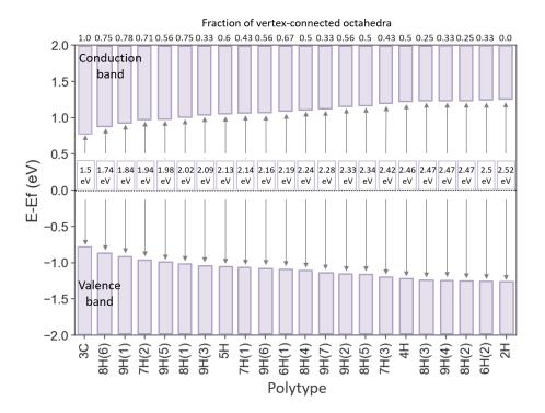
Figure 6. Energy level scheme for APbI<sub>3</sub> polytypes from DFT calculations without SOC.
