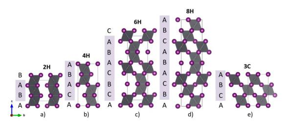
Figure 1. The topology of experimentally known APbX<sub>3</sub> close-packed polymorphs accordingly [2] and [3]: (a) 2H, (b) 3C − cubic structure is shown in hexagonal axes, (c) 4H, (d) 6H, (e) 8H.
