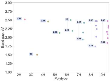
Figure 3. The strip plots of the calculated band gap from the number of close-packed layers in polytypes. Color dots show the value of the calculated band gap without SOC for a particular polytype. The numbers show the maximum and minimum calculated values of the band gap for the polytypes with the same close-packed.
