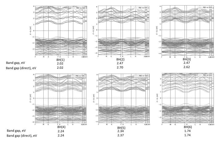
Figure S7. Calculated band structure without SOC for possible 8H polytypes of APbI<sub>3</sub>.
