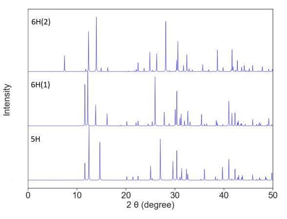
Figure S9. Calculated XRD pattern for 5H and 6H polytypes.
