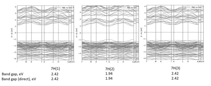
Figure S6. Calculated band structure without SOC for possible 7H polytypes of APbI<sub>3</sub>.
