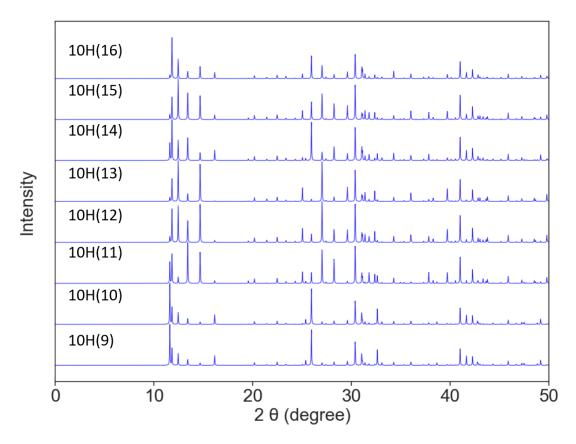
Figure S13b. Calculated XRD pattern for 10H (9-16) polytypes.
