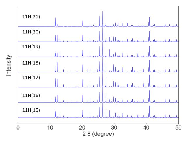
Figure S14c. Calculated XRD pattern for 11H (15-21) polytypes.
