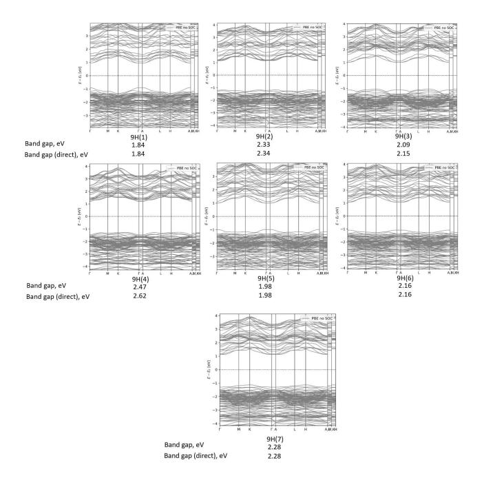
Figure S8. Calculated band structure without SOC for possible 9H polytypes of APbI<sub>3</sub>.
