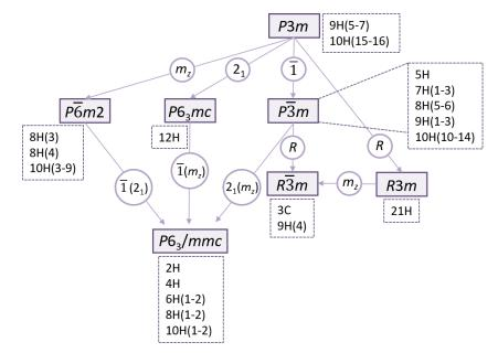
Figure 2. Symmetry relationships between undistorted close packings of ABX<sub>3</sub>. The dotted line shows the symmetry of polytype packings with the number of layers (n) from 2 to 10. Space group *P*6<sub>3</sub>*mc* occurs for the first time among 12H and *R*3*m* among 21H polytypes. The numbers in parentheses indicate the serial numbers of the polytypes.
