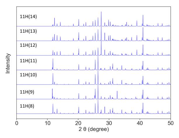
Figure S14b. Calculated XRD pattern for 11H (8-14) polytypes.
