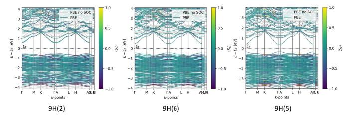
Figure S3. The band structures of 9H polytypes with different proportion of *h* and *c* close-packed layers. Gray color shows calculations without SOC, color shows results of calculations with SOC.
