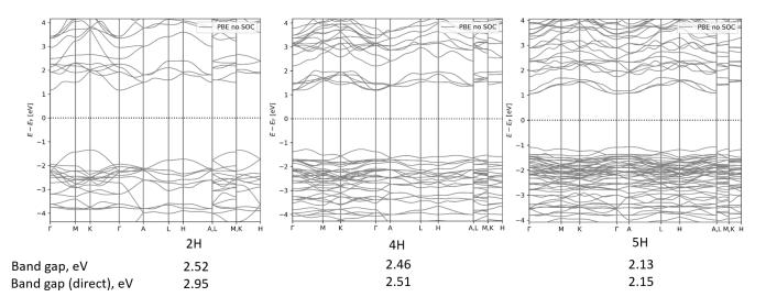
Figure S4. Calculated band structure without SOC for possible 2H, 4H and 5H polytypes of APbI<sub>3</sub>.
