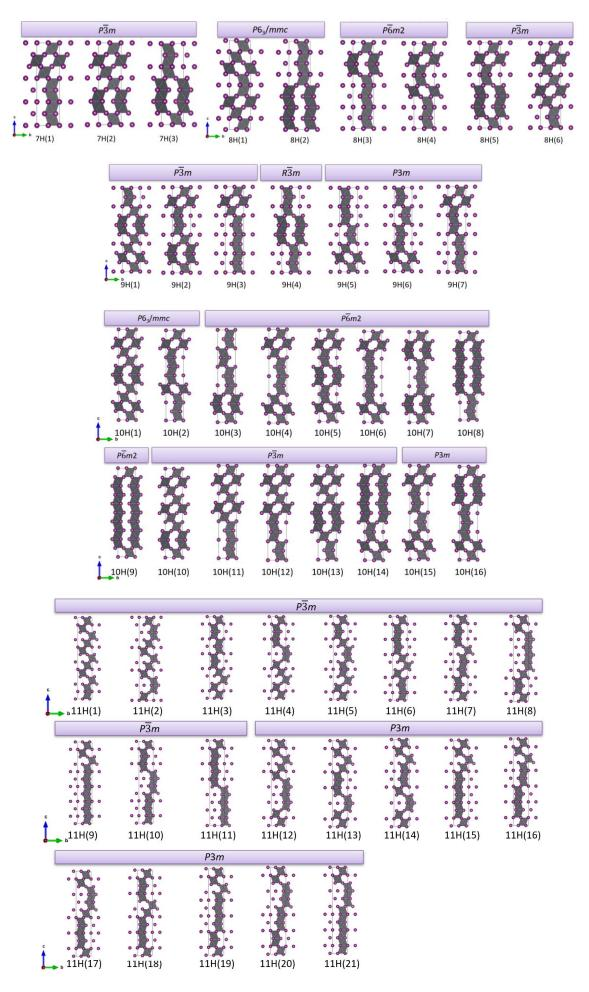
Figure S1. Constructed all possible 7H, 8H 9H, 10H and 11H close-packed polytypes of APbI<sub>3</sub>.
