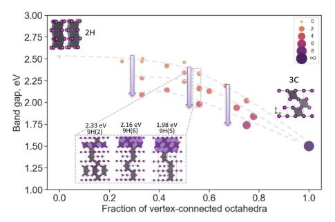
Figure 5. The band gaps and proportions of vertex-connected Pbl<sub>6</sub> octahedra in hexagonal polytypes with 2-9 close-packed layers. The size of the balls shows the size of the «cubic» block of vertex-connected octahedra in the crystal structure of polytype.
