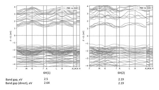
Figure S5. Calculated band structure without SOC for possible 6H polytypes of APbI<sub>3</sub>.
