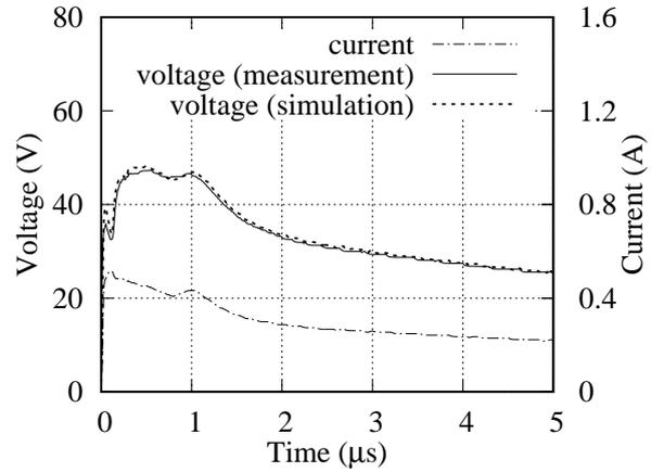
Figure 5: Measured and calculated ground potential rise.
