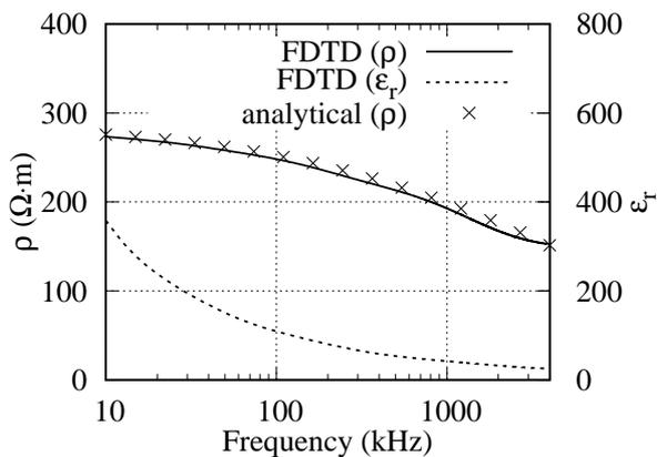
Figure 10: Apparent soil properties calculated with different methods.
